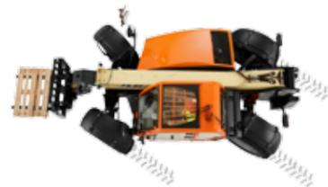
Crab steer for sideways movement and precise positioning before lifting.
